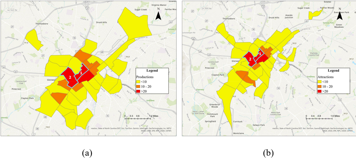
(a) (b) Figure 10: Number of (a) Productions and (b) Attractions by Census Block Group
